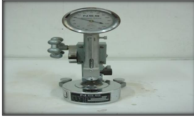
Fig. 4: The device used to determine the surface hardness values of manufactured specimens.
