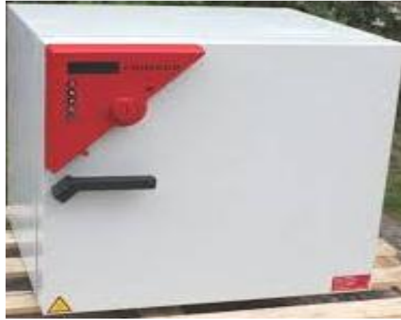
Fig. 3: Image of the electric oven used to expose models to the thermal physical effect.
